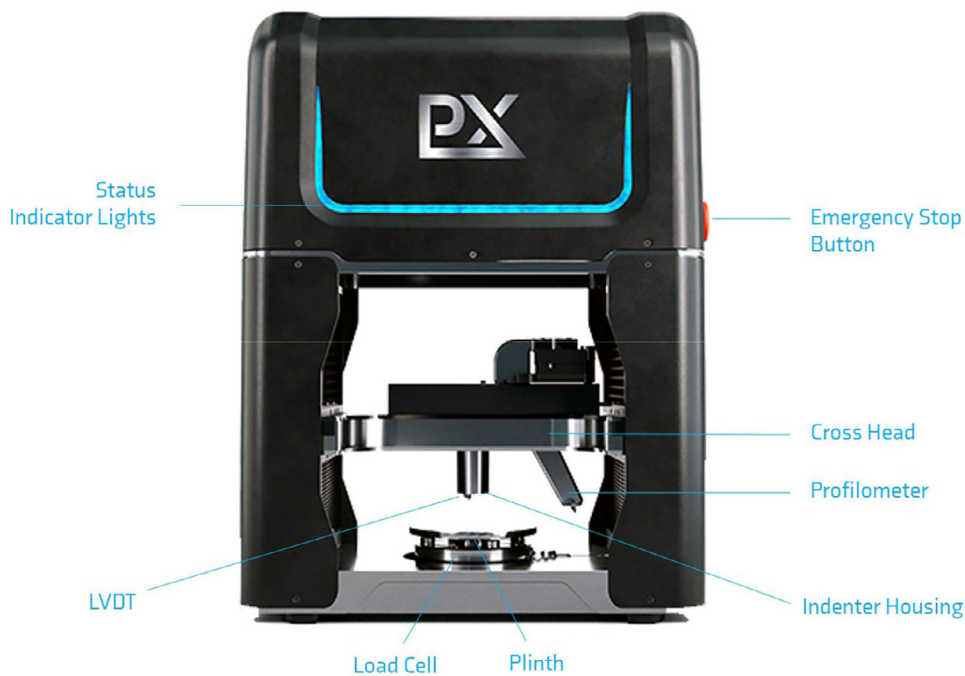
Fig. 2. Image of the Plastometer, with the key components labeled.
