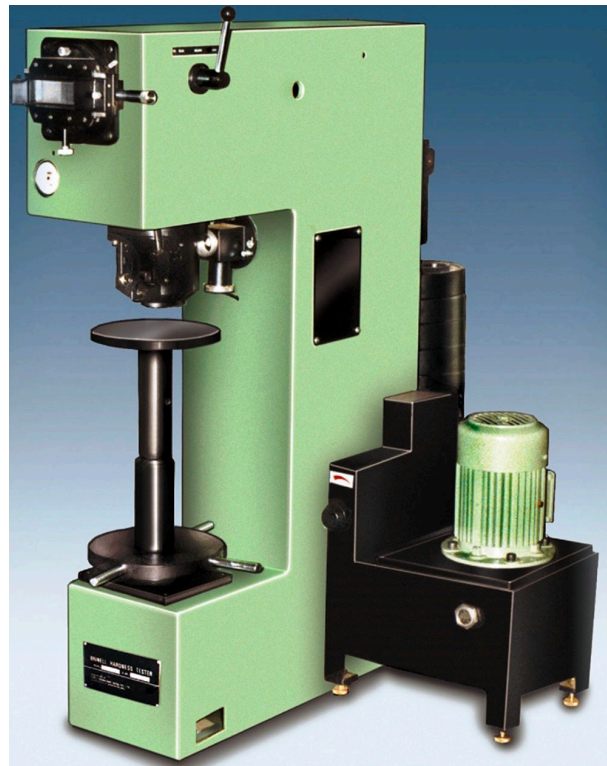
Fig.1 Photo of a typical Brinell hardness testing facility.
