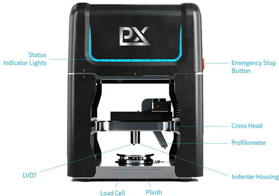
Figure 7. Image of the PLX Plastometer, with the key components labeled.
